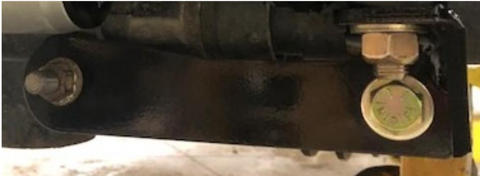
The passenger side outer shock mount attaches to the tie rod with the OEM bolts that held the OEM shock bracket in place.
