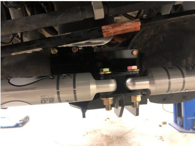
Locate the shocks and tie plate. Use the 1/2 x 2 1/2" bolts to fasten the body end of the shocks to the K bracket. The tie plate goes on top. The shaft end of the shocks attach to the outer shock mounts with the 1/2 x 2 1/2" shocks.
