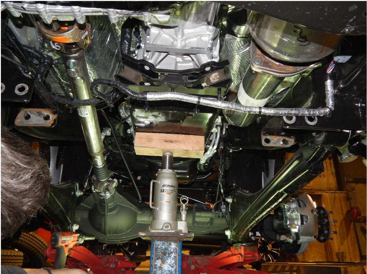
3. Locate the crossmember (Part # 18291). It fastens into the factory crossmember holes with the four 5/8 x 6 1/2" bolts. Also use the M18 x 40 bolts to fasten the side of the crossmember into the original control arm mounts. Torque these bolts to 150 ft./lbs. Now locate the three factory transmission nuts and fasten them to the crossmember. Torque to 40 ft/lbs.
