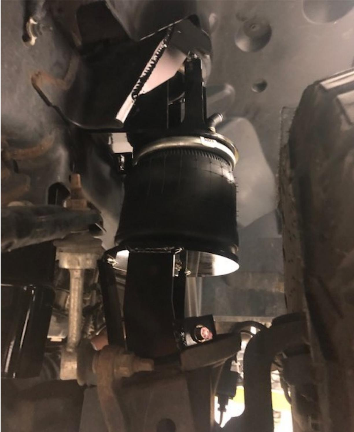
*NOTE: The passenger side upper spring bucket has a gusset welded on from the factory. The drivers side doesn't have this bracket. A weld in bracket is supplied for the drivers side. Once you have the air bag installed, wrap up the air bag and mounts and weld the gusset in place. Do not place the gusset too close to the air bag or it will rub on it. Once you have this mount welded in, paint it black to match the chassis.*
