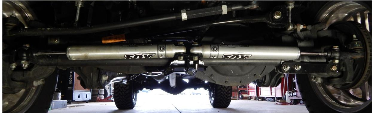
15. Locate the sway bar drops (Part # 18336DS and 18314PS). Fasten in place with the factory bolts on the top and fasten the sway bar to the sway bar drop with the 7/16 x 1 1/2" bolts. Torque to 50 ft./lbs.
