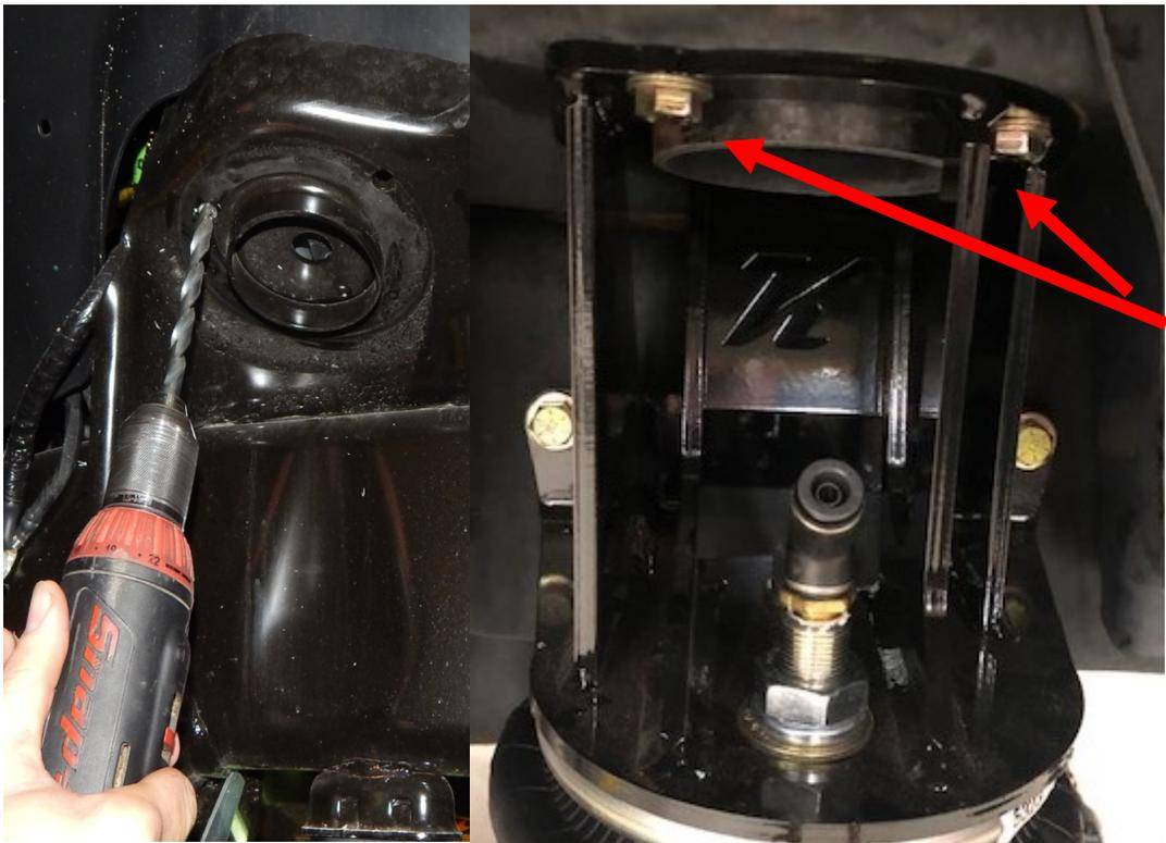
*Drill and tap these two holes in the side of the frame*
