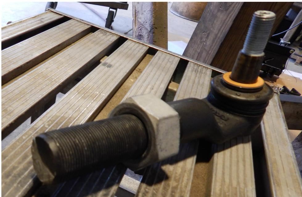
6. Locate the dropped pitman arm (Part # 4011). Remove the factory pitman arm and replace with the dropped one. Torque the nut to 275 ft./lbs. Rotate the ball joint on the end of the steering arm 180 degrees as it will go into the pitman arm from the bottom up now. Insert the ball joint into the pitman arm and torque the steering arm nut on the ball joint to 100 ft./lbs. NOTE: The pitman arm needs to be re-torqued after 300 miles.
