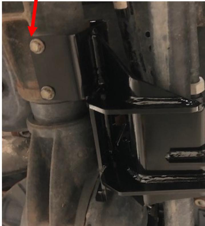
14. Locate the center plate (Part # 20227 ), shocks (Part # Fox 985-24-068) and outer shock mounts (Part # 1840PS and 18389/18409DS). The driver side outer shock mounts fasten to the tie rod with the OEM bolt and the 1/2 x 2 1/2" bolt.
