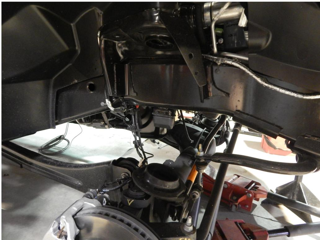
2. Place a jack under the transfer case. Remove the three nuts from the transmission mount where it fastens to the crossmember and remove the four bolts that hold the transmission crossmember in place. Remove the crossmember. Remove the two bolts that fasten the control arms to the frame. Keep the nuts for the transmission mount. The other bolts will not be used.
