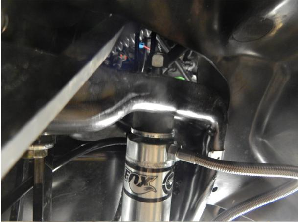
12. Place a bushing over the shock shaft so the large ring is down. Install the washer dish down. Thread on the lock nut until it bottoms out. Fasten the remote reservoirs to mounts. If using Fox brand shocks, use the hose clamps. If using the Kelderman shocks, use the billet clamps.
