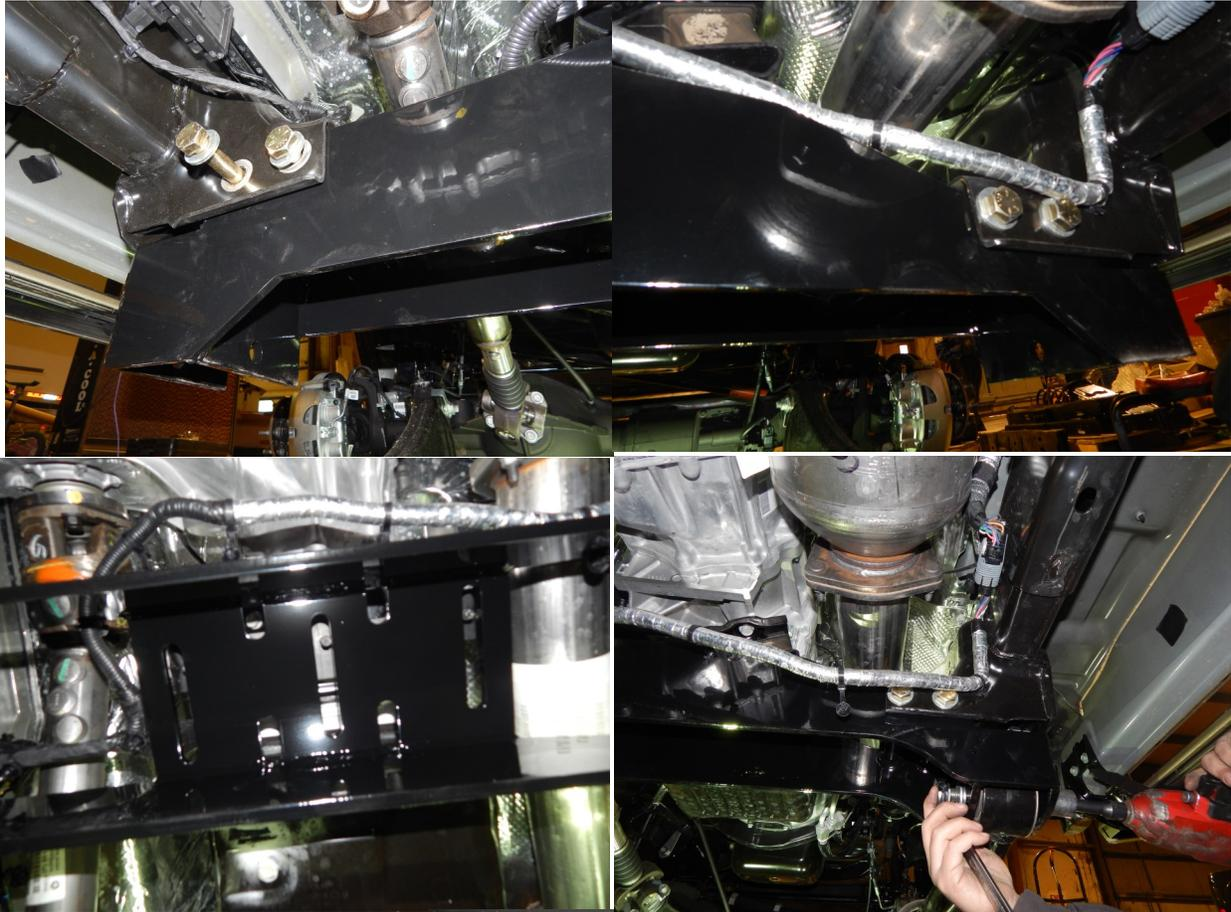
4. Fit the factory control arms into the new crossmember. Use the supplied M18x140 bolts. Insert them from the outside in and torque to 150ft/lbs.
