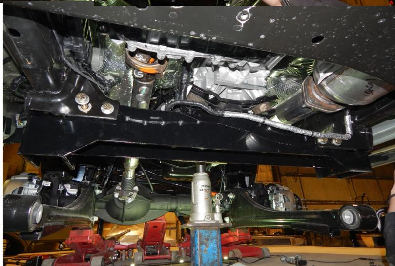
5. Remove the ball joint from the steering linkage. The tab needs to be cut off so the ball joint can be turned 180 degrees over and installed into the new pitman arm that gets installed in the next step.
