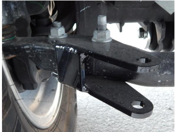
3. Locate the drivers side bracket (part# 18839 and 18397) If fastens to the two factory pinch bolts on the steering arm. It also fastens to the outer tie rod end with the 1/2x3" bolts. Torque these bolts to 55 ft/lbs. Make sure the 1/2" bolt is pointing towards the rear of the truck.
