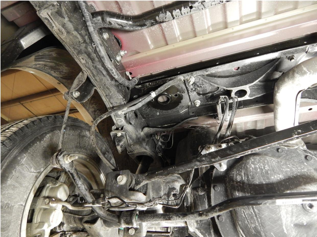
3.) Locate the upper air bag mounts (part # XXXXDS and XXXXPS). They fasten into the upper coil mounts with the 1/2" and 3/4" nut mounts (Part # 19113 and 19114). Fasten the upper bag mounts in place and torque the 1/2" bolts to 85 ft./lbs. and the 3/4" bolts to 125 ft./lbs. NOTE: The cut out for the air line fitting on the drivers side faces towards the center of the truck and the cut out on the passenger side faces towards the front/and passenger side frame rail.
