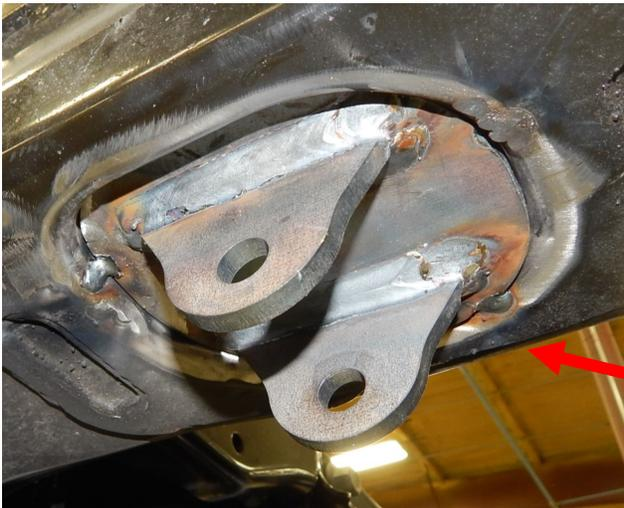
13.) With the shock mounts are installed, locate the shocks (Part # 10095 Raptor) and install. Use the xx bolts on top and OEM 14mm bolts on the bottom to fasten into place. Torque the bolts to 95 ft./lbs.
