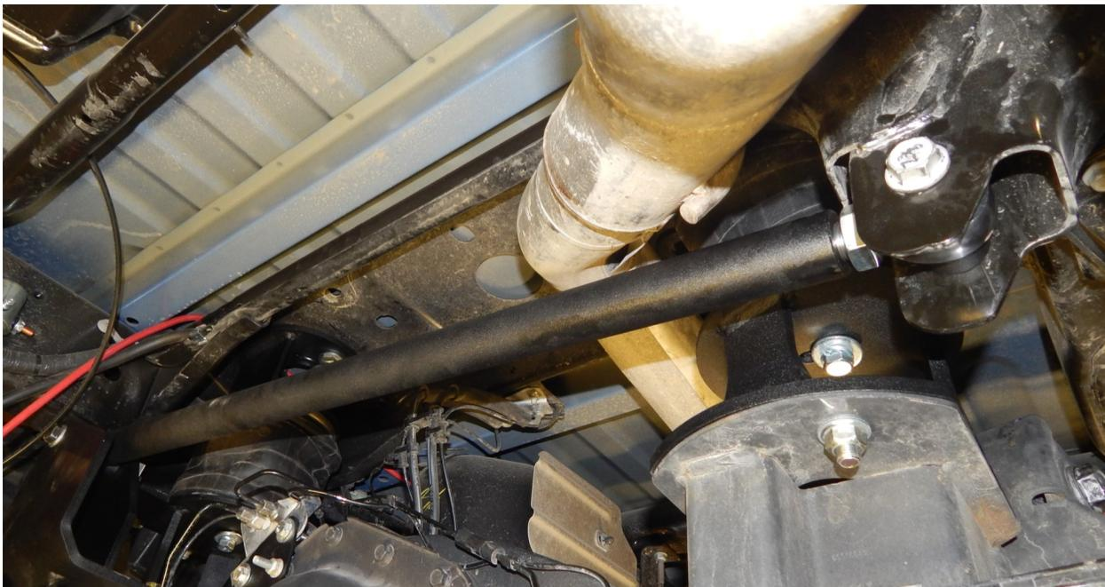
9.) Locate the two holes in the top of the coil spring perch. Use a 17/32" drill bit to open up the holes. Locate the passenger side lower bag mount (Part # xxx) and fasten to the axle with the two 1/2 x 1 1/2" bolts. Torque to 85 ft./lbs.
