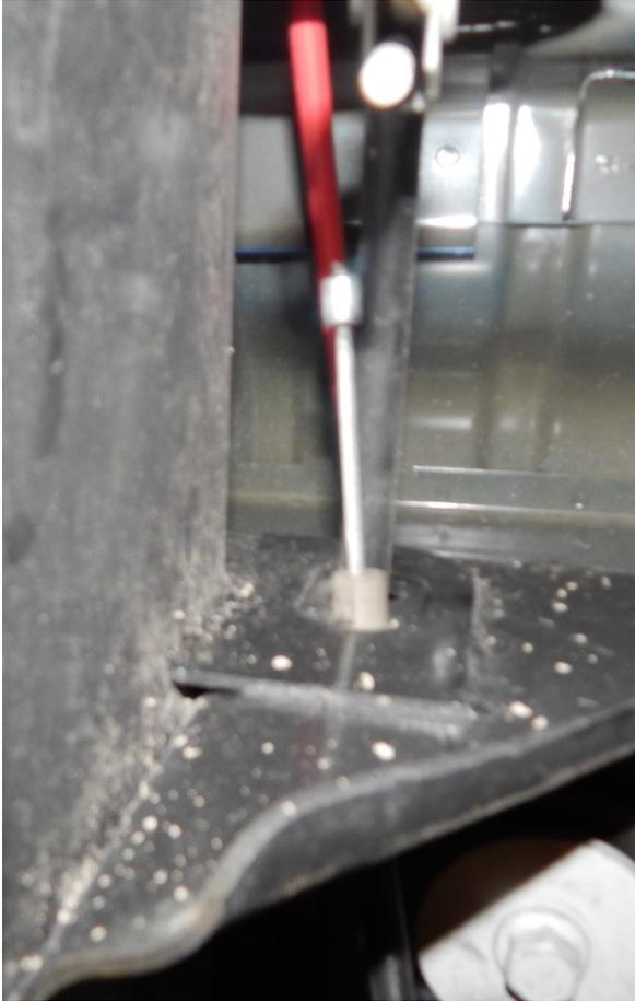
6.) Remove the drivers side e-brake cable from the metal loop that holds it in place. Unhook it from the connection on the side of the frame and push it back through the mounting brackets. It will now drop down and run up to the forward bracket. It will also tie into the lower forward trailing arm knuckle pinch bolt with the supplied clamp.
