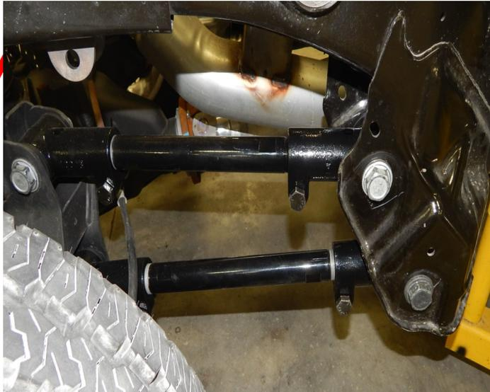
7.) Locate the lower bag mounts (Part # xxxx DS and xxxxPS). Beginning with the driver side, place the bag mount on the axle. It fastens with the three 1/2 x 1 1/2" bolts (one hole gets drilled) and the factory panhard bar bolt into the factory panhard bar mount. Once all the bolts are installed, torque the 1/2" bolts to 85 ft./lbs. and the factory panhard bar bolt to 120 ft./lbs.
