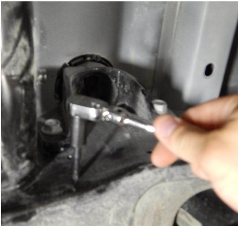
3. Use a center punch to locate where to drill. Once you center punch hold the height control valve back in position to make sure your center punch marks are accurate. Next drill the two 3/16" holes. Once the holes are drilled tap the holes with a 1/4-20" tap.
