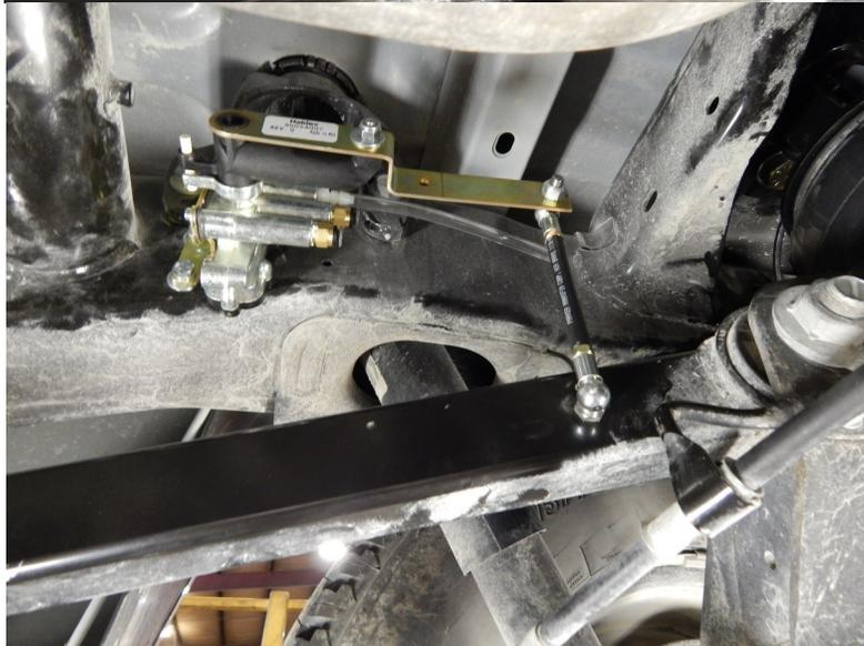
5. The linkage should be 5 1/4" long. Double check that the air bags are at 8" (measure in between the mounting brackets). Now use a center punch and mark your drill location. Drill the hole with a 1/4" drill bit. Next tap the hole with a 5/16-18 tap. Install the ball and linkage. Look closely at the linkage and you will see a wire "keeper". Remove the keeper, slide the linkage on and install the rod on the balls. Reinstall the keepers.
