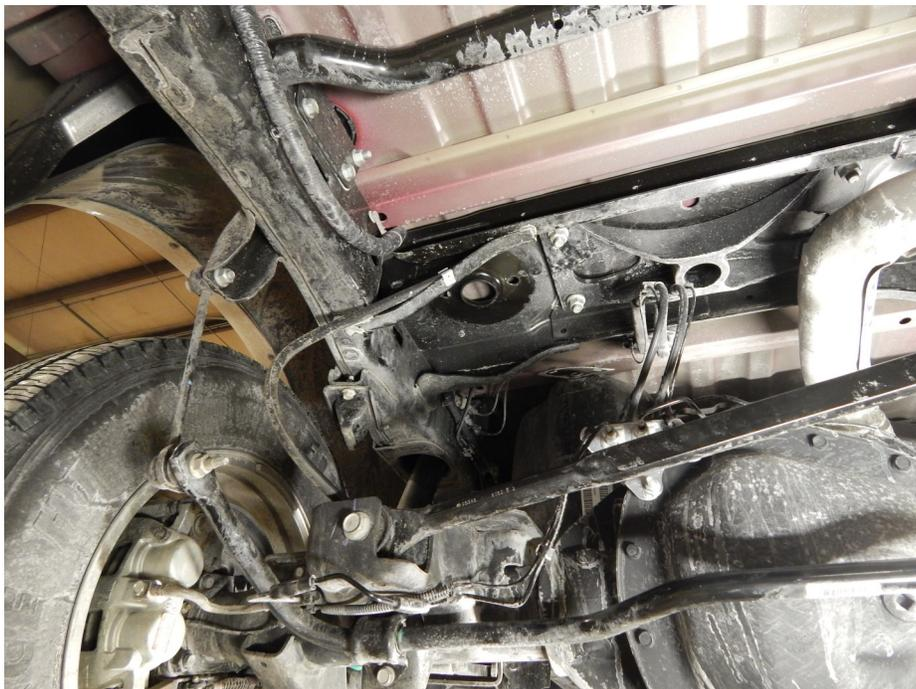
2. Locate the upper air bag mounts (part# 19106-DS and 19107-PS). They fasten into the upper coil mounts with the 1/2" and 3/4" nut mounts (Part # 19113 and 19114). Fasten the upper bag mounts in place and torque the 1/2" bolts to 85 ft./lbs. and the 3/4" bolts to 125 ft./lbs.
