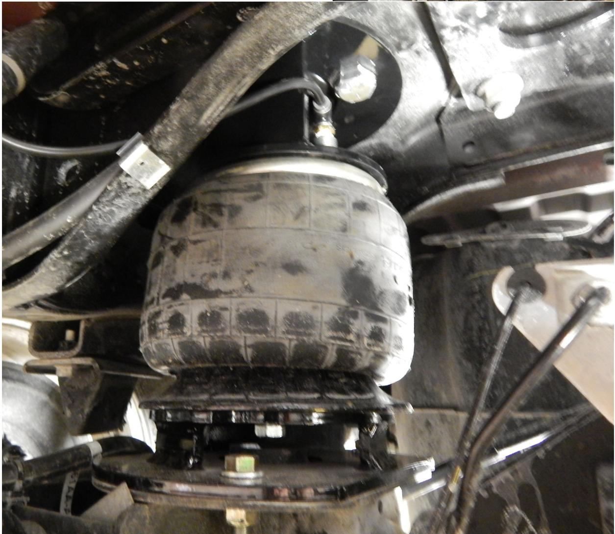
7. The ride height of the 5323 air bags is 8". Measure between the upper and lower air bag mounts. If you are using the wireless remote control set up, use the instructions supplied with the kit. If you are using the electronic self leveling kit, you will need to use those instructions. Steps 9 & 10 will show the mounting position of the rear sensors. The front sensors are also shown in these instructions on page 8.
